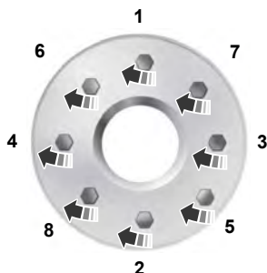
8-lug nut torque sequence
