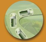
Ford's AdvanceTrac® with RSC® (Roll Stability Control™) features unique functionality thanks to a second gyroscopic roll rate sensor to determine the vehicle's body roll angle and roll rate. If the unique roll rate sensor detects a significant roll angle, the system applies additional countermeasures — such as applying brakes to one or more wheels or reducing engine power — to enhance vehicle rollover resistance.
