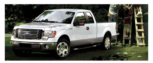
The 2010 Ford F-150 rises to the challenge of tough jobs, featuring a fully boxed frame constructed with hydroformed and high-strength steel side rails for increased durability and safety. The sturdy chassis also delivers class-leading towing and hauling capability across all cab configurations, while still returning fuel economy of 15 mpg city/21 hwy on 4x2 models with the 4.6-liter 3V V-8 engine.
