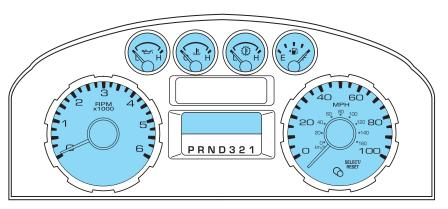
**Speedometer:** Indicates the current vehicle speed.
