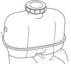
The fluid level will drop slowly as the brakes wear, and will rise when the brake components are replaced. Fluid levels between the MIN and MAX lines are within the normal operating range; there is no need to add fluid. If the fluid levels are outside of the normal operating range, the performance of your brake system could be compromised; seek service from your authorized dealer immediately.
