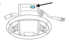
2. Apply the brake. Use a tool (or a small screwdriver) to pry out the access cover. Insert the tool into the access hole and slide the white override button towards the left. Move the gear shift lever into N (Neutral) while holding the white override disc towards the left.
