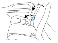
To gain access to the storage compartment in your armrest, lift the latch to open the lid. The lid cannot be opened in the upright position.
