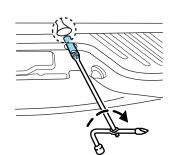
5. Remove the retainer through the center of the wheel.
