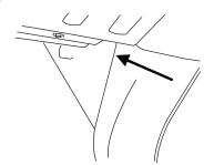
To remove the fuse panel cover, pull the panel toward you. When the clips of the panel disengage, let the panel fall easily.
