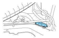
3. Partially lower tailgate and carefully feed tailgate harness up through the gap between the pickup box and the bumper. Place the tailgate harness out of the way under the pickup box.
