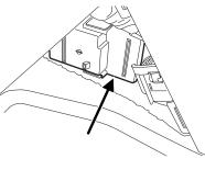
To remove a fuse use the fuse puller tool provided on the fuse panel cover.
