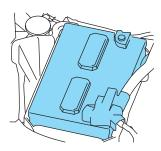
Your vehicle is equipped with a Motorcraft® maintenance-free battery which normally does not require additional water during its life of service.
