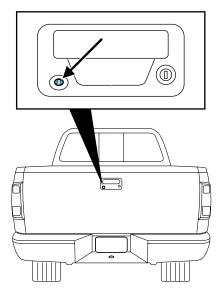
To use the camera system, place the transmission in R (Reverse); an image will display on the left portion of the rearview mirror or on the navigation screen (if equipped). The area displayed on the screen may vary according to the vehicle orientation and/or road condition.
