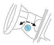
4. Turn the hazard flashers on then off 3 times. This must be accomplished within ten seconds.
