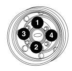
4. Be sure to install all the clips on the nuts over the flanges so that there is an even gap all around and the retention clips are fully seated.
