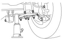
13. Insert the jack handle into the pump linkage.
