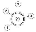
2. Turn ignition from the 3 (on) position back to the 1 (off) position in order to remove the first **coded key** from the ignition.
