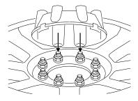
If the ornament retention towers are aligned between the studs/lug nuts, the ornament is improperly installed. This improper installation may appear and sound correct, but will not keep the ornament on the vehicle. Ornaments improperly installed in this manner will fall off or become loose with minimal force or impact.
