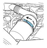
2. Carefully separate the two halves of the air filter housing.
