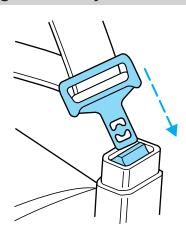
5. To put the retractor in the automatic locking mode, grasp the shoulder portion of the belt and pull downward until all of the belt is extracted and a click is heard.
