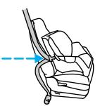
4. Insert the belt tongue into the proper buckle (the buckle closest to the direction the tongue is coming from) for that seating position until you hear and feel the latch engage. Make sure the tongue is latched securely by pulling on it.
