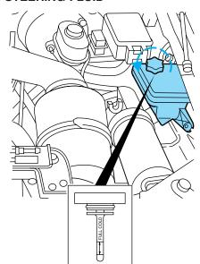
Check the fluid level when it is at ambient temperature,  $20^{\circ} - 80^{\circ}$  F (-7° - 25° C):
