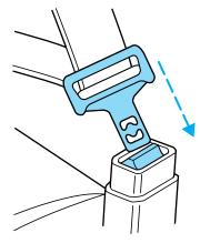
• Grasp the shoulder portion and pull downward until the entire belt is extracted.
