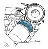
4. Install a new air filter element, ensuring the arrow on the top half of the air filter housing lines up with the notch on the bottom half of air filter housing. Be careful not to crimp the filter element edges between the air filter housing. This could cause filter damage and allow unmetered air to enter the engine if not properly seated.
