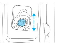
Move lock control up to engage the childproof lock. Move control down to disengage childproof locks.
