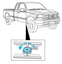
3. Fluid level should be at bottom of the opening.
