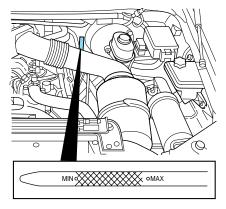
6. Wipe the indicator clean. Insert the indicator fully, then remove it again.
