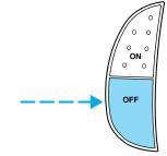
Once speed control is switched off, the previously programmed set speed will be erased.
