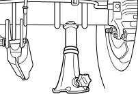
8. Turn the jack handle clockwise until the wheel is completely off the ground and high enough to install the spare tire.
