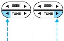
• Press to select the next disc in the CD changer. Hold the control to fast-forward through the remaining discs.
