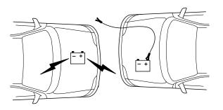
1. Connect the positive (+) booster cable to the positive (+) terminal of the discharged battery.
