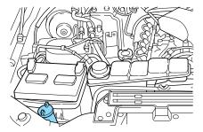
Only use a washer fluid that meets Ford specifications. Refer to *Lubricant specifications* in the *Capacities and specifications* chapter.
