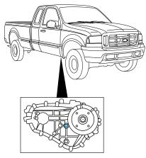
3. Add only enough fluid through the filler opening so that the fluid level is at the bottom of the opening.
