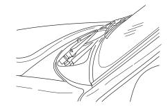
• Do not place objects over the defroster outlets. These objects can block airflow and reduce your ability to see through your windshield. Also, avoid placing small objects on top of your instrument panel. These objects can fall down into the defroster outlets and block airflow and possibly damage your climate control system.
