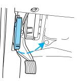
2. Go to the front of the vehicle and release the auxiliary latch located under the right center of the hood. Slide the handle to release the auxiliary latch.
