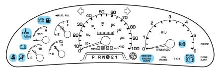
Make sure the corresponding lights illuminate briefly. If a light fails to illuminate, have the vehicle serviced.
