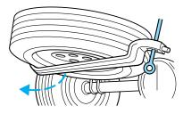
3. If equipped, unlock and remove the spare tire lock from the rear bumper drive tube using the the spare tire lock key and the jack handle.
