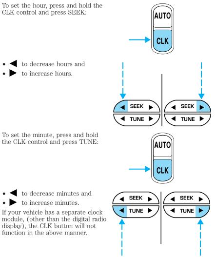
The CLK button will allow you to switch between media display mode (radio station, stereo information, etc.) and clock display mode (time). When in clock mode, the media information will display for 10 seconds, when the radio is turned on, and then revert to clock information. Anytime that the media
