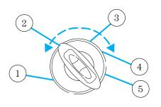
4. ON, all electrical circuits operational. Warning lights illuminated. Key position when driving.
