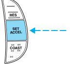
• Accelerate with your accelerator pedal. When the desired vehicle speed is reached, press and release SET/SET ACC/SET ACCEL.
