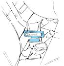
• Insert the belt tongue into the proper buckle until you hear a snap and feel it latch. Make sure the tongue is securely fastened in the buckle.
