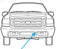
For best results, plug the heater in at least three hours before starting the vehicle. Using the heater for
