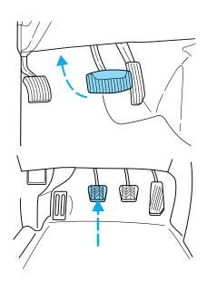
• Depress the clutch pedal (if equipped).
