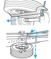
5. Remove the retainer through the center of the wheel.
