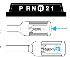
**Drive** – Not shown on the display. Activate by pressing the Transmission Control Switch (TCS) on the end of the gearshift lever with the gearshift in the **①** position. The TCIL (the word OFF) will illuminate on the gearshift lever. Transmission operates in gears one through three. **①** (Drive) provides more engine braking than **①** (Overdrive) and is useful when:
