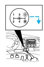
With the 6-speed transmission you can shift into R (Reverse) by moving the gearshift left from N (Neutral).
