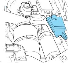
5. If the fluid is low, add fluid in small amounts, continuously checking the level until it reaches the range between the ADD/MIN and MAX lines. Be sure to put the cap back on the reservoir.
