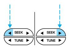
To set the minute, press and hold the CLK control and press TUNE:
