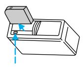
Make sure only one disc is inserted in each slot. Each disc must be inserted with the label surface upward. Depending on your system, you may insert up to six or ten CDs.
