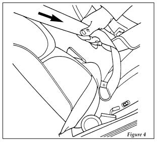
Setting the retractor to automatic locking mode
