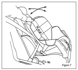
Checking that the seat is secure
