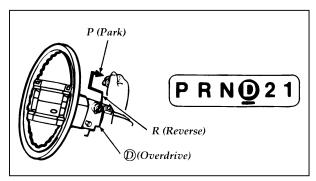
The positions of the column-mounted gearshift
