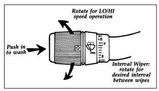
Interval wiper on turn signal lever
