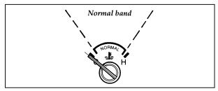
Engine coolant temperature gauge
