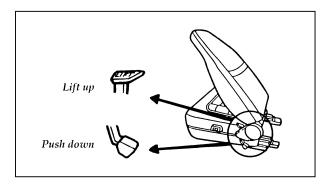
Prior to operating the vehicle, check to ensure that the seat assembly is locked by pushing or pulling the seat forward or rearward. If seat does not lock, repeat steps 2 and 3.
