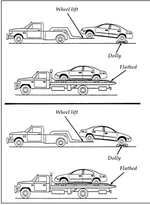
When calling for a tow truck, tell the operator what kind of vehicle you have. A towing manual is available from Ford Motor Company for all authorized tow truck operators. Have your tow truck driver refer to this manual for the proper hook-up and towing procedures for your vehicle.
