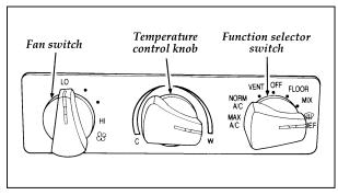
Climate control knobs (Heater A/C system)
