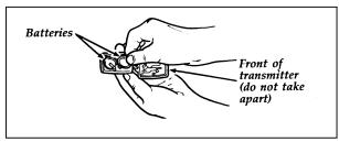
**Replacing the batteries**
