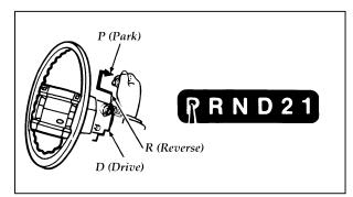
The positions of the column-mounted gearshift
