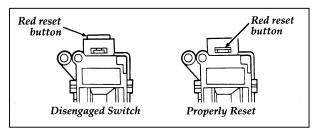
Reset button for fuel pump shut-off switch
