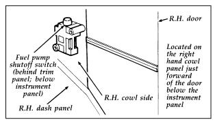
Fuel pump shut-off switch location
