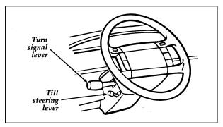
Turn signal and tilt release wheel lever
